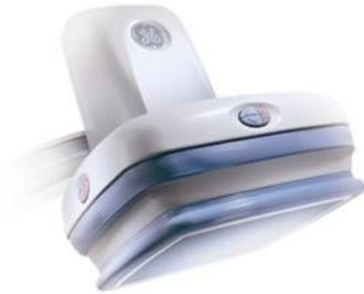
The GE digital detector on the Innova 3100<sup>IQ</sup> system replaces the entire imaging chain of a traditional X-ray image intensifier system. By converting X-ray signals into digital images at the point of acquisition, the detector captures information with minimal loss over the full range of typical exposures to produce exceptional image clarity. It also minimizes the artifacts and distortions associated with conventional X-ray systems.
